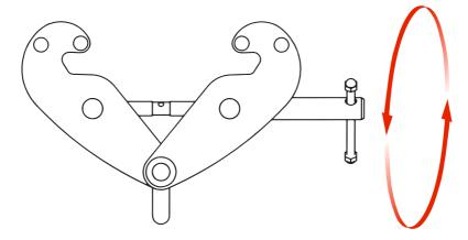
Loads are attached to the forged eye and must be central to the clamp.
